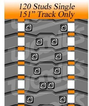
The Long Track Template 114 single pattern is used to create this 120 stud pattern. Read Tech Tip T7-12-0012
