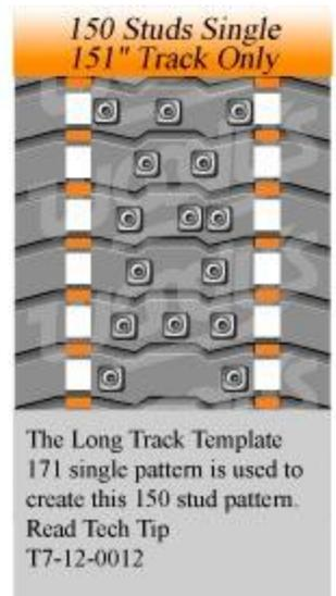
To create this 150 stud pattern – 1<sup>st</sup> template placement mark X's and W's. 2<sup>nd</sup> template placement mark Y's and Z's. **Omit marking the center most location every other pitch for a 3-2-3-2-3-2 pattern.**
